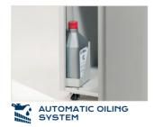
Automatically lubricates the cutting knives during the shredding operation. ensuring maximum reliability, efficiency and capacity.
