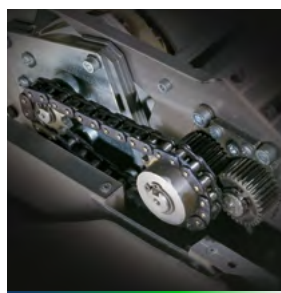
Chain drive with steel gears.
