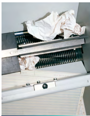
Automatic mechanical feeding system utilizes revolving flaps to feed material into cutting knives.
