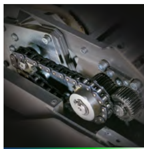
Chain drive with steel gears.
