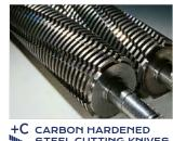
STEEL CUTTING KNIVES accept staples and metal clips.
