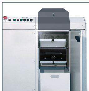
Easy access to cutting units and waste container
