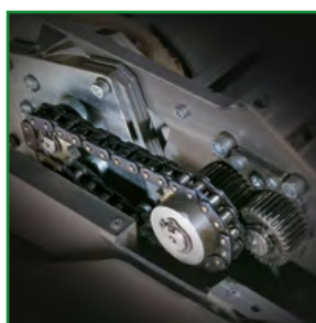
Chain drive with steel gears.
