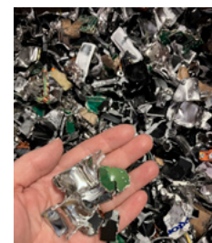
Easy removal and emptying of waste container. Particles of size \leq 2000 \text{ mm}^2 (H-4).
