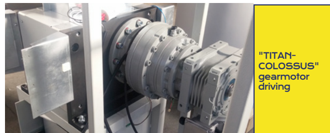
The Kobra HDD is equipped with the "Titan-Colossus" gearmotor driving specially designed heavy duty cutting knives with unmatched power to shred large quantities of rotational and digital media devices, including: Hard Disk Drives up to 3.5", Solid State Drives (SSD), LTO, Ultrium magnetic tapes and Solid State Devices (Phones and PDAs).
