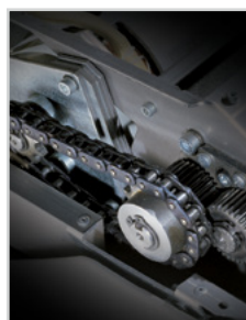
SUPER POTENTIAL POWER SYSTEM: chain drive system with steel gears.
