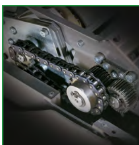
Chain drive with steel gears.
