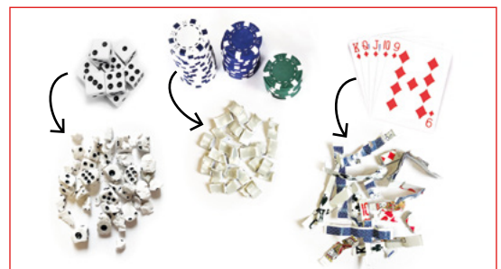
Shredded material samples: 12,5 x 20 mm dices and poker chips shreds, 12,5 x 20-88 mm playing cards shreds.
